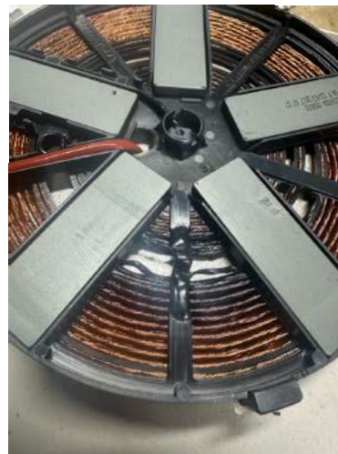
Coil overheating and burn out.
